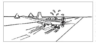
Proper crosswind technique is a must. In the case of a left crosswind, the left wing must be lowered into the wind and this control input countered with right rudder to maintain the proper track down to the runway. Again, the longitudinal axis of the airplane must be aligned with the flight path which, we hope, is parallel to the runway centerline.
